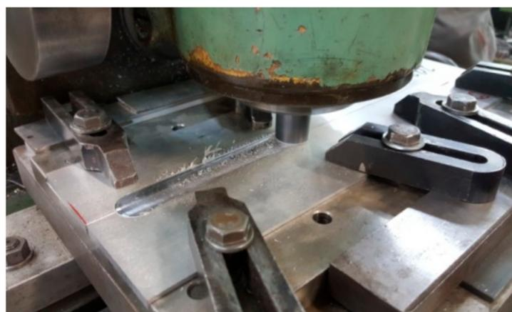
**Figure 1.** Conventional Milling Machine for friction stir welding (FSW).
