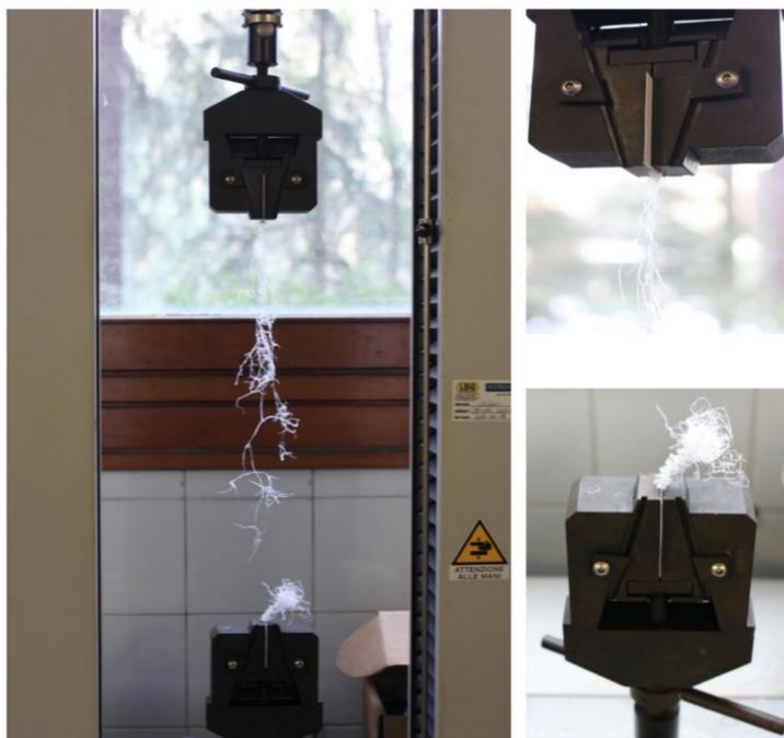
Figure 6. Typical tensile failure of the composite.
