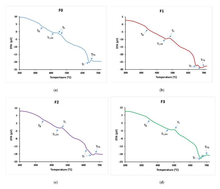
Figure 3. Differential scanning calorimetry curves of (a) F<sub>0</sub>, (b) F<sub>1</sub>, (c) F<sub>2</sub>, and (d) F<sub>3</sub>.
