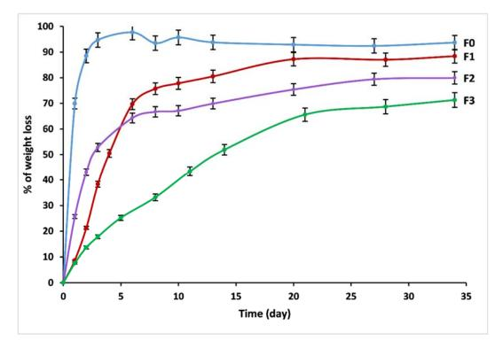
**Figure 7.** Trend of weight loss of F<sub>0</sub>, F<sub>1</sub>, F<sub>2</sub> and F<sub>3</sub> glasses.
