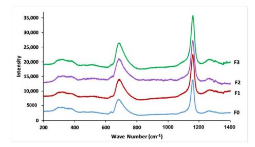
Figure 5. Raman spectra of prepared glasses.
