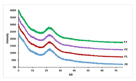
Figure 2. XRD patterns for F<sub>0</sub>, F<sub>1</sub>, F<sub>2</sub> and F<sub>3</sub> glasses.
