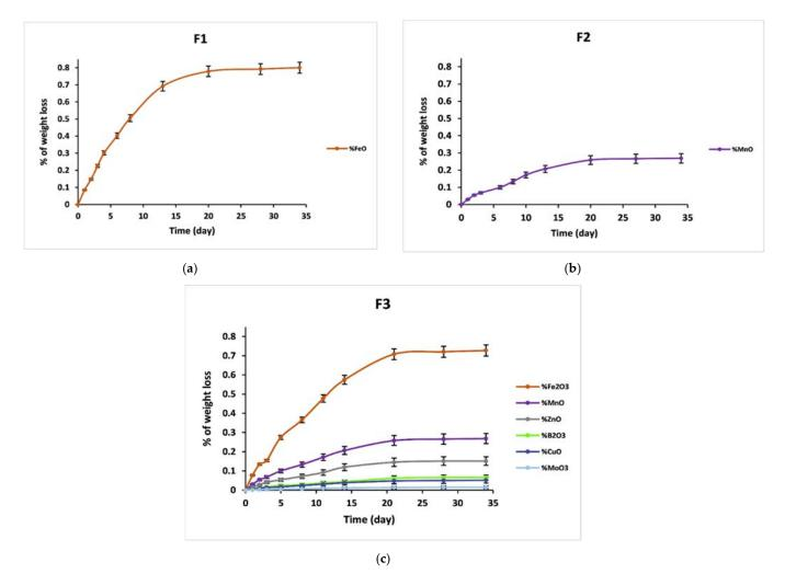
**Figure 9.** Percentage of glass constituents (micro-elements) analyzed in the leachate solutions (elements in the form of oxides) normalized to the initial glass weight for (**a**)  $F_{1,r}$  (**b**)  $F_{2,r}$  and (**c**)  $F_{3}$ .
