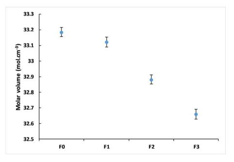
Figure 4. Molar Volume of F<sub>0</sub>, F<sub>1</sub>, F<sub>2</sub>, and F<sub>3</sub> glasses.
