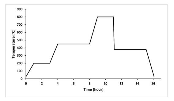
Figure 1. Thermal profile used to elaborate glasses.
