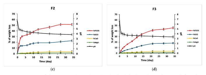
**Figure 8.** Percentage of glass constituents (macro-elements) analyzed in the leachate solutions (elements in the form of oxides) normalized to the initial glass weight and pH measurements versus time for (**a**)  $F_0$ , (**b**)  $F_1$ , (**c**)  $F_2$ , and (**d**)  $F_3$ .
