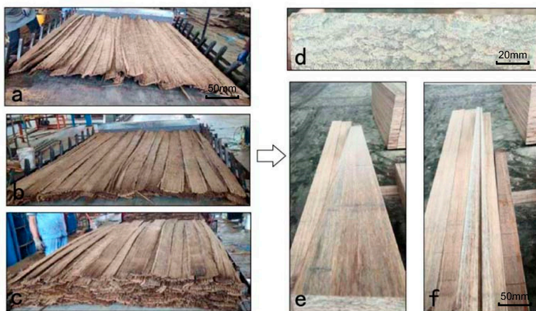
Figure 2. Bamboo fiber composite (BFC) formation: (a) first layer on caul plate, (b) mat build-up showing strips with minimal overlap of core strips, (c) finished lay-up, (d) cross-section of consolidated panel and (e,f) re-sawn billets from a BFC panel.
