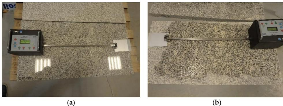
**Figure 7.** Dynamic coefficient of friction measurement: (a) PO series in dry condition, (b) flamed (PL) series in wet condition.
