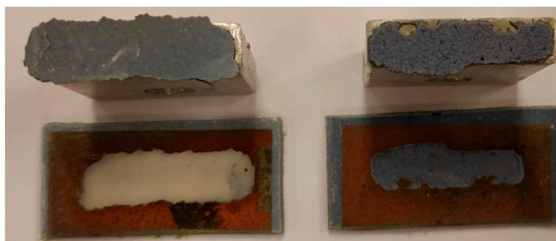
**Figure 9.** Sample photos of metallized coatings with compound B and stamps after the pull off test.
