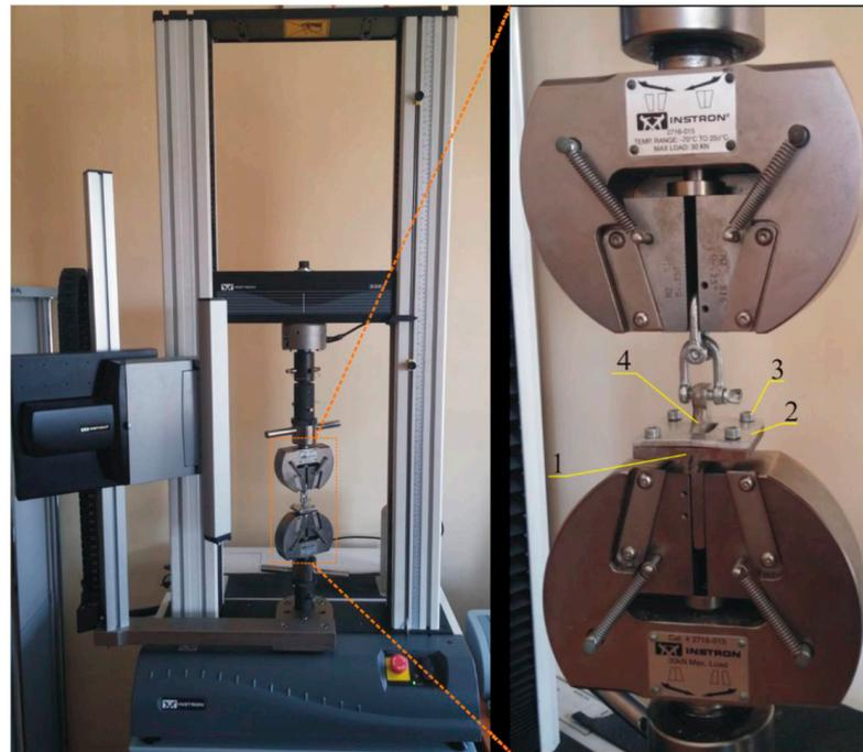
**Figure 1.** The clamps for testing the adhesive strength of coatings and deposited copper layers; the tested sample was mounted between the fixed base (1) and the cover (2) by clamping with screws (4), with a hole for a punch (4) in the cover (2).
