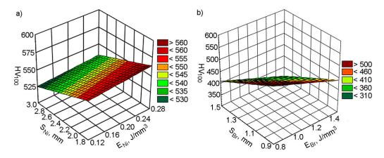
**Figure 4.** The effect of the energy density and laser spot pitch on the microhardness of the deposited tracks: (a) nickel-based alloy; (b) bronze.
