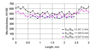
**Figure 7.** Changes in microhardness in the cross section of three neighboring deposited tracks under a laser spot speed of  $V_{Ni}/V_{Br}$  = 120/200 mm/min and different pitches.
