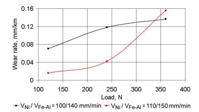
**Figure 10.** The dependence of the linear wear rate of the composite coating on a load under boundary lubrication conditions.
