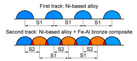
Figure 1. The composite coating deposition scheme.
