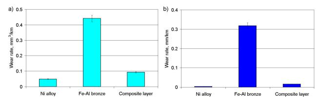
Figure 11. Comparing the wear rates under various friction conditions. (a) Dry friction, (b) boundary friction.
