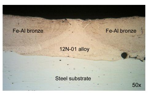
**Figure 2.** The fragment of coating deposited under conditions: laser spot speeds  $V_{\text{Ni}}/V_{\text{Br}} = 160/250 \text{ mm/min}$  and laser spot pitches  $S_1/S_2 = 2.4/1.2 \text{ mm}$ .
