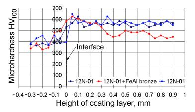
**Figure 5.** The distribution of micro-hardness by the depth of the coating layer, deposited under conditions  $V_{Ni}/V_{Br} = 120/200 \text{ mm/min}$  and  $S_1/S_2 = 2.4/1.2 \text{ mm}$ .
