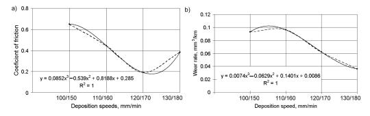
**Figure 9.** The dependence of the CoF (**a**) and the wear rate (**b**) of the composite coating under dry friction conditions on the deposition speed (dotted line—empirical data, solid line—approximation equation).
