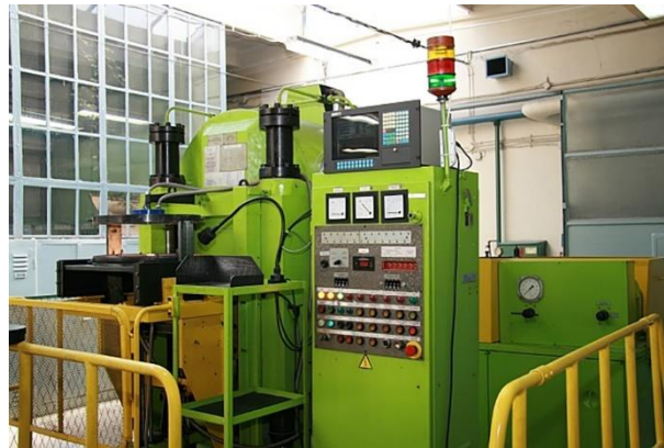
Figure 5. Device for high pressure spark plasma sintering [133].
