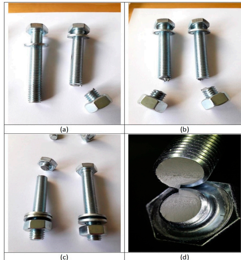
Figure 10. Bolt failure: (a) failure of one bolt at nut location; (b) failure of both bolts at nut location; (c) failure of one bolt at head location; (d) appearance of the fracture surface.
