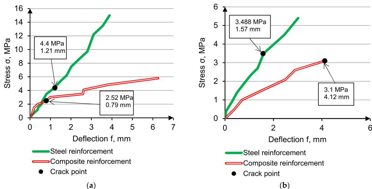
Figure 12. Stress-deflection curves for LWC D1600 concrete 3 (a), D1000 concrete 4 (b), reinforced by steel and composite.
