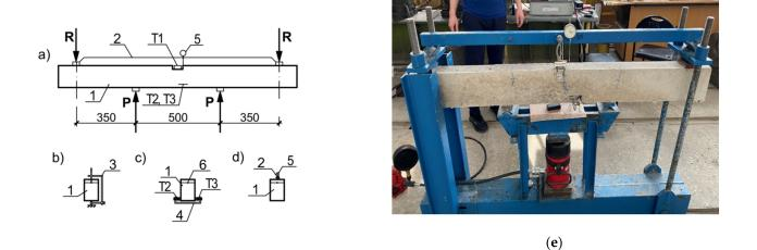
**Figure 4.** Beam testing scheme. (a) load and device placing; (b) strain gauges T1 fixing; (c) strain gauges T2, T3 fixing; (d) deflection indicator fixing; 1—beam; 2—deflection measurement traverse; 3, 4—strain gauges T2, T3 fixing; 5, 6— deflection indicator; (e) beam testing photo.
