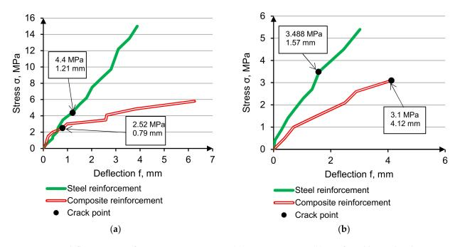
Figure 12. Stress-deflection curves for LWC D1600 concrete 3 (a), D1000 concrete 4 (b), reinforced by steel and composite.
