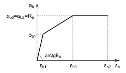
Figure 5. Three-line concrete deformation diagram.
