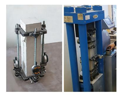
Figure 1. Concrete sample modulus of elasticity under compression testing.
