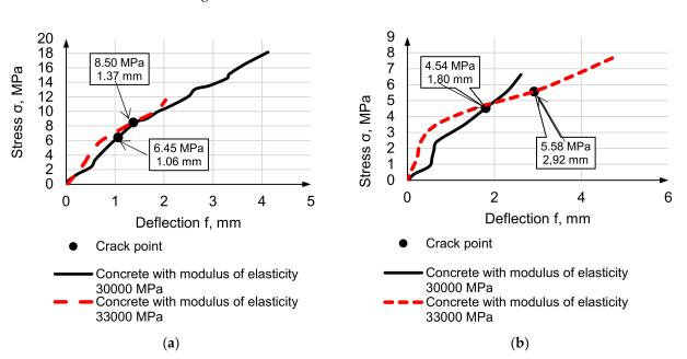
3.2. Research of Concrete Sample Beams Reinforced by Steel and Composite under Bending Tensile
