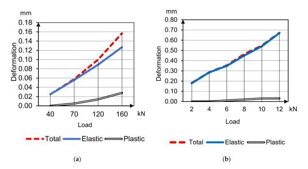
Figure 6. Deformation and deflection curves for concrete 1 under compression (a) and bending (b) tensile.
