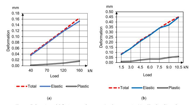
Figure 7. Deformation and deflection curves for concrete 2 under compression (a) and bending (b) tensile.
