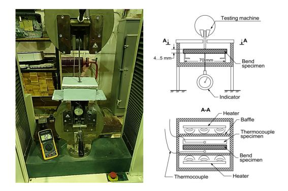
Figure 3. The three-point bending test rig.
