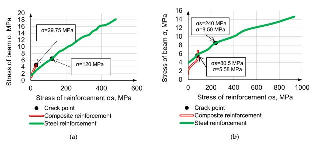
concrete with high-modulus steel reinforcement. Cracking point stress of lightweight concretes decreases accordingly to elasticity modulus decreasing but not to strength. Beam stress-reinforcement stress curves are presented in Figure 13.
