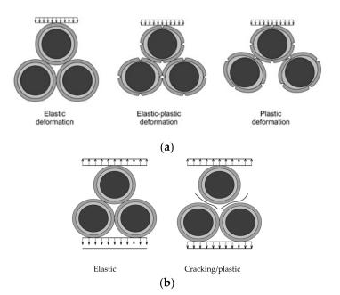
**Figure 10.** Stages of concrete deformations until destruction. (**a**) under compression three stages, (**b**) under tensile two stages.
