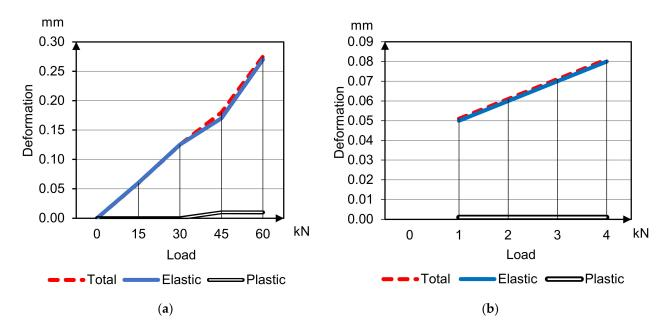
Figure 8. Deformation and deflection curves for concrete 3 under compression (a) and bending (b) tensile.
