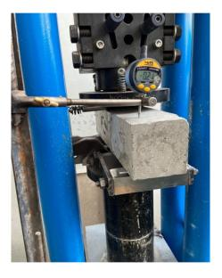
Figure 2. Bending tensile testing scheme 1—loading element; 2—beam sample; 3—support.
