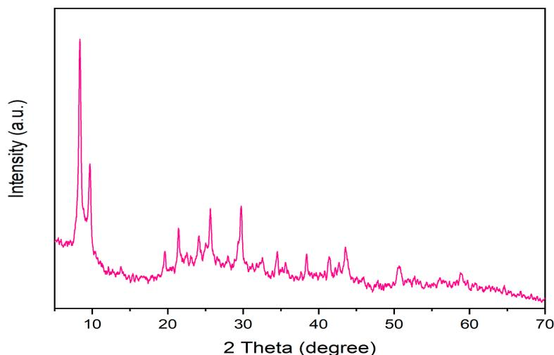
Figure 1. PXRD diffraction patterns of dry and soaked prepared Bio-MOF (MIP-202).
