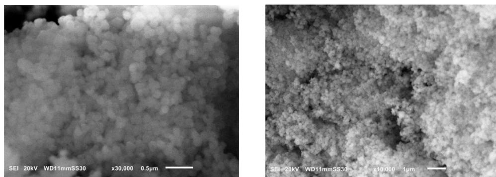
**Figure 6.** SEM images at different magnifications of the prepared Bio-MOF (MIP-202), synthesized at 110 °C for 18 h in pure water.
