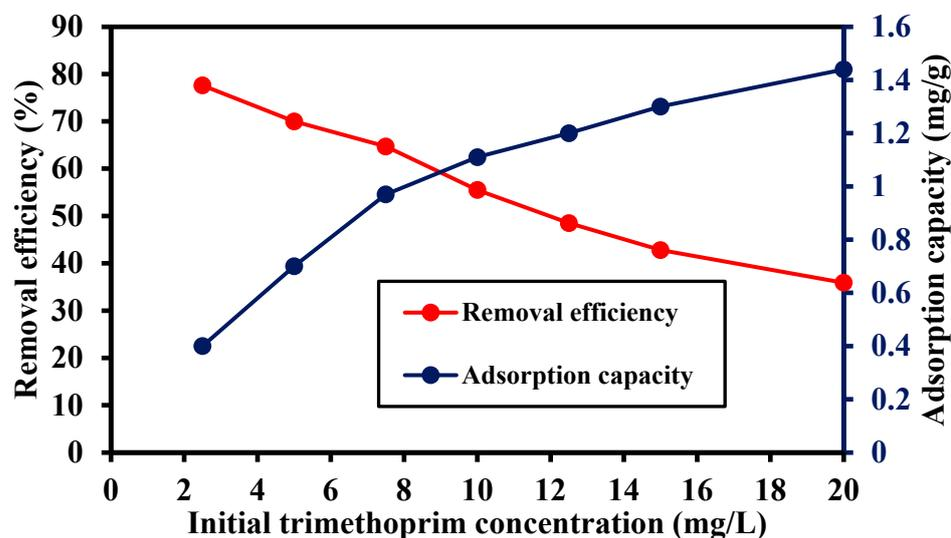
**Figure 8.** Effect of initial trimethoprim concentration on the removal efficiency of trimethoprim antibiotic and the adsorption capacity of Bio-MOF, pH of 7, contact time of 60 min, and adsorbent dose of 0.5 g/L.
