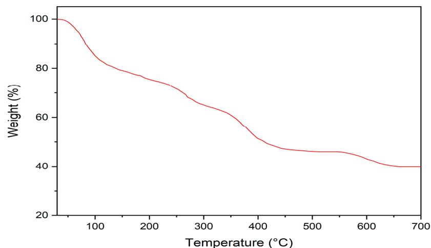
Figure 3. TGA profile of the prepared Bio-MOF (MIP-202).
