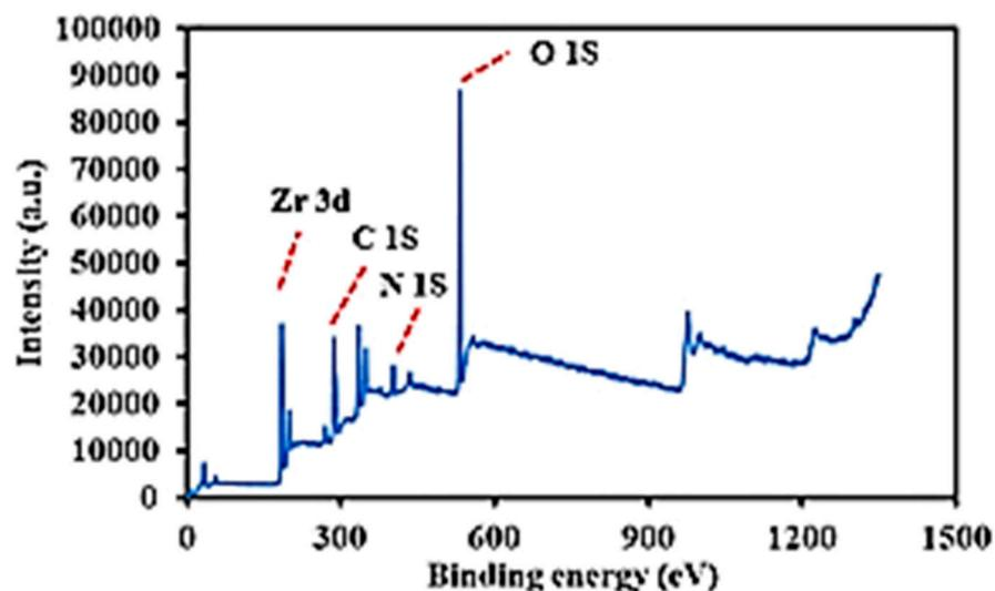
**Figure 5.** XPS analysis of the prepared Bio-MOF (MIP-202).
