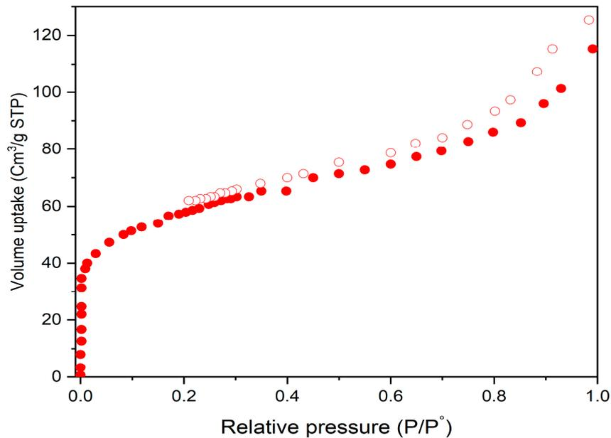
**Figure 4.**  $\text{N}_2$  adsorption–desorption isotherms for the BET surface area of the prepared Bio-MOF (MIP-202).
