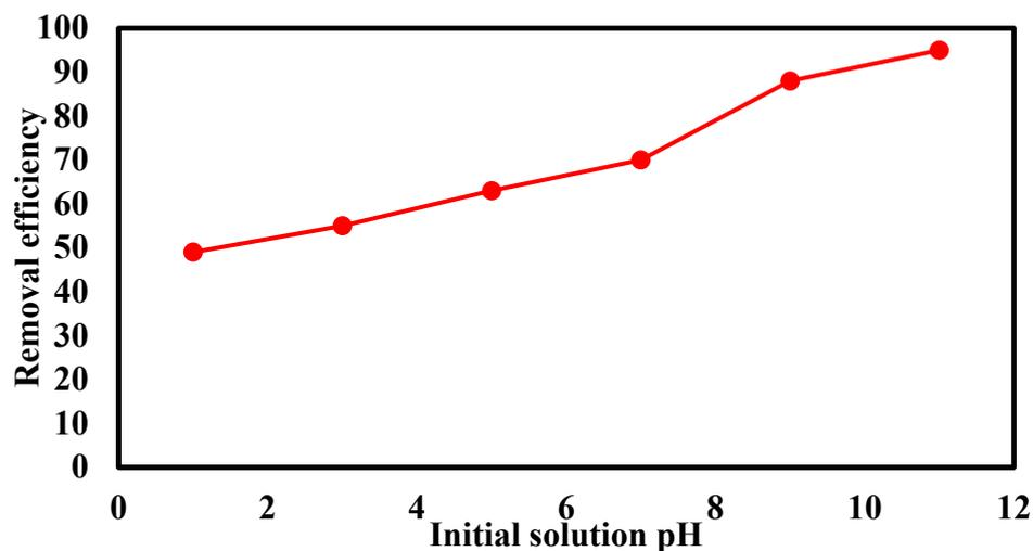
Figure 10. Effect of solution pH on the removal efficiency of trimethoprim antibiotic, contact time of 60 min, and adsorbent dose of 0.5 g/L.
