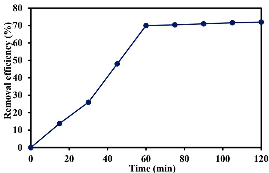
**Figure 7.** Effect of contact time on the removal efficiency of trimethoprim antibiotic at pH of 7, initial trimethoprim concentration of 10 mg/L, and adsorbent dose of 0.5 g/L.
