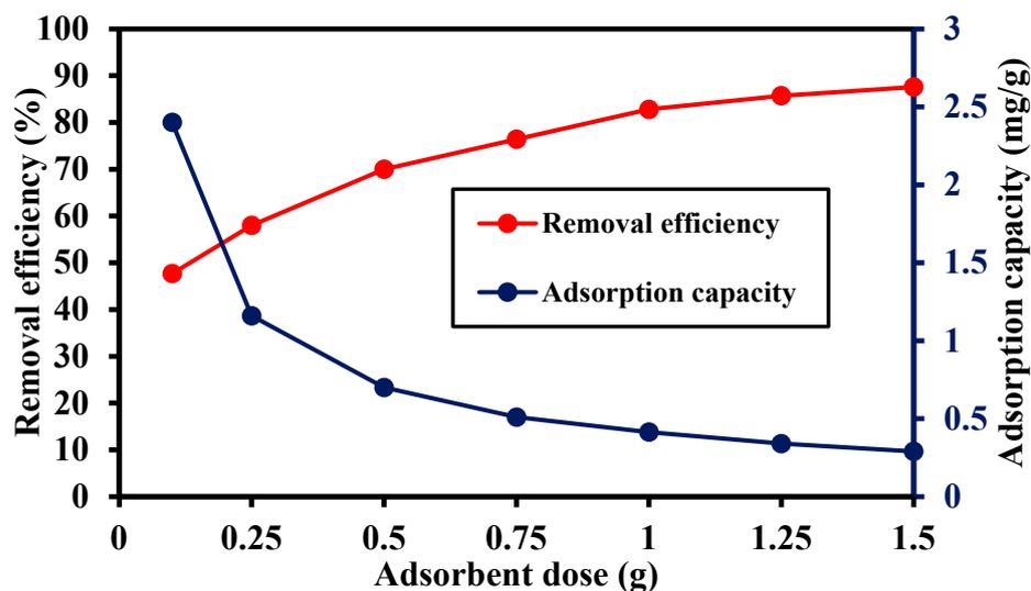
Figure 9. Effect of adsorbent dose on the removal efficiency of trimethoprim antibiotic and the adsorption capacity of Bio-MOF, pH of 7, contact time of 60 min, and adsorbent dose of 0.5 g/L.
