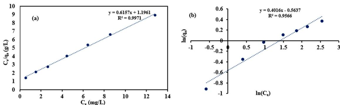
**Figure 11.** The linear adsorption isotherms of the trimethoprim antibiotic onto Bio-MOF: (a) Langmuir model and (b) Freundlich model.
