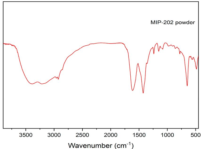
Figure 2. FTIR spectra of prepared Bio-MOF (MIP-202).
