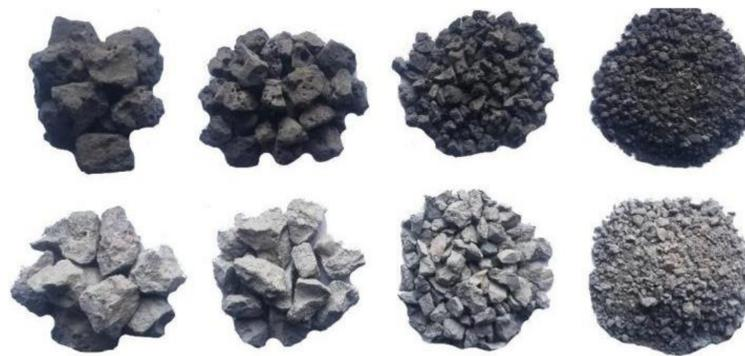
**Figure 4.** Steel slag and concrete-recycled macadam with different particle sizes.
