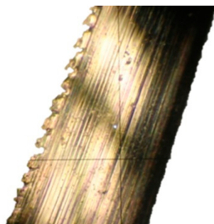
Figure 19. View of the chip shape after longitudinal turning without coolant (36 HRC).
