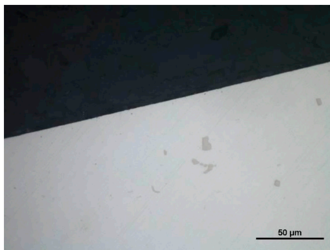
Figure 27. A view of a microsection after longitudinal turning with cooling and before etching.
