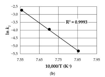
**Figure 12.** (a)  $\ln k_1$  against temperature (b)  $\ln k_2$  against temperature employing first-order kinetic model rate constants of decay plotted in Arrhenius form.
