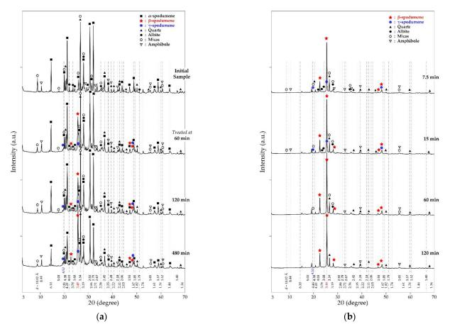
**Figure 9.** XRD patterns of residues obtained after concentrate treatment in air as a function of residence time at 900  $^{\circ}$ C (a) and 1050  $^{\circ}$ C (b).
