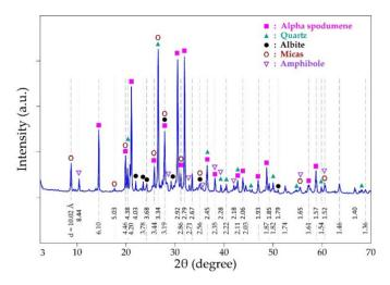
Figure 2. XRD patterns of spodumene concentrate.
