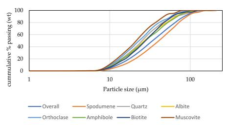
Figure 3. Mineral particle size determined by MLA.
