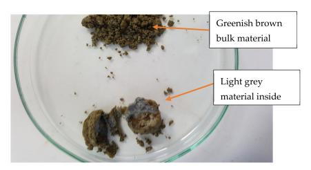
Figure 1. Optical image showing both the bulk and grey material contained in agglomerate particles.
