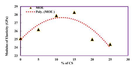
Figure 7. Modulus of elasticity of CS Concrete.
