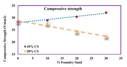
Figure 9. The compressive strength of concrete contains different ratios of FS and CS.
