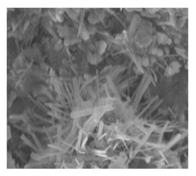
Figure 17. Coconut shell replacement of in concrete (15%).
