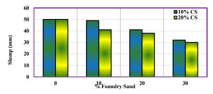
Figure 8. Slump test results.
