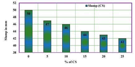
Figure 3. Slump of CS concrete.
