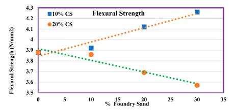
Figure 10. Flexural strength of concrete contains various ratios of FS as well as CS.
