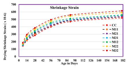
Figure 14. Drying shrinkage strain contains different percentages of FS and CS.
