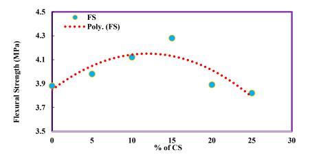
Figure 6. Flexural strength of CS concrete.
