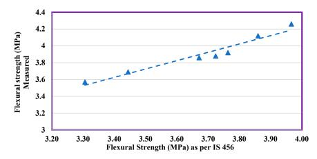
Figure 12. Measured flexural stress vs. computed flexural strength.
