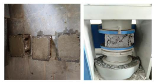
Figure 2. Casting and testing of CS concrete specimen.
