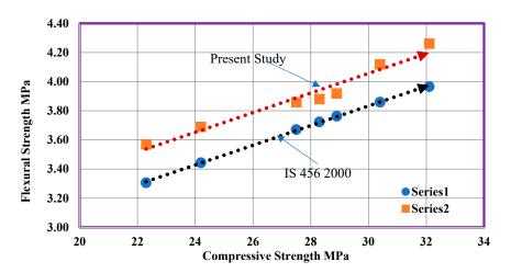
**Figure 11.** A study of flexural strength and compressive strength of concrete, containing different percentages of FS as well as CS.
