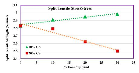
Figure 13. Split tensile strength contains various percentages of FS as well as CS.
