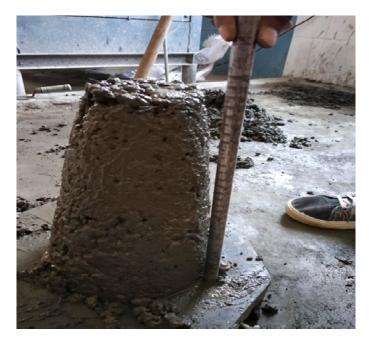
Figure 1. Slump of CS concrete.
