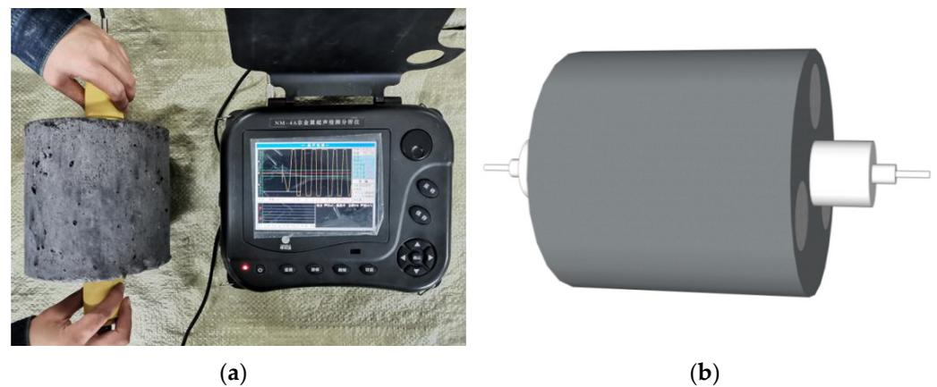
**Figure 6.** (a) Ultrasonic test and (b) simulation diagram of the ultrasonic test.
