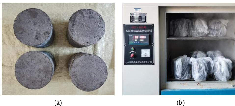
**Figure 4.** (a) Prepared specimens and (b) curing of specimens.
