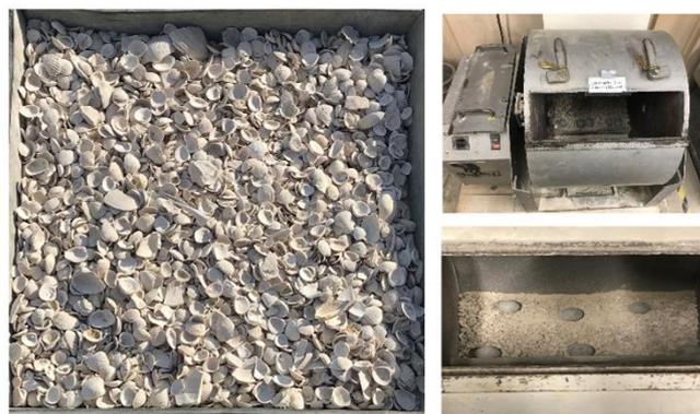
Figure 1. Florida washed shell before and after crushing.
