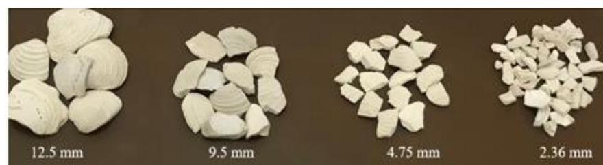
Figure 2. Florida washed shell particles of various sizes used in this study.
