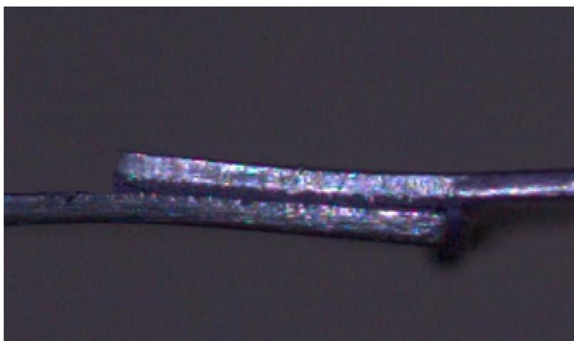
**Figure 13.** Representative image of the plastic deformation to which the mild steel substrates were subjected during the SLJ tests.
