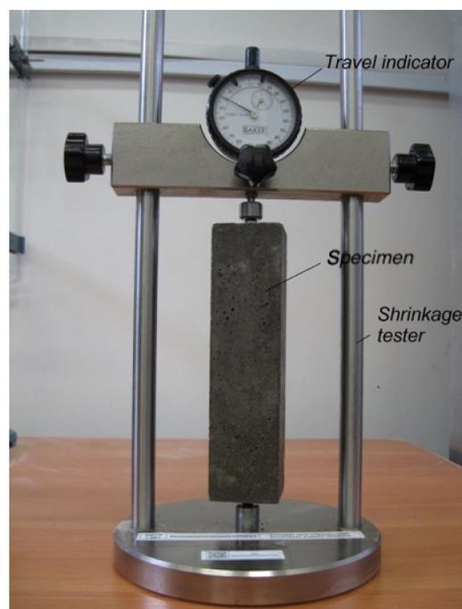
**Figure 3.** Device for measuring shrinkage of concrete specimens.
