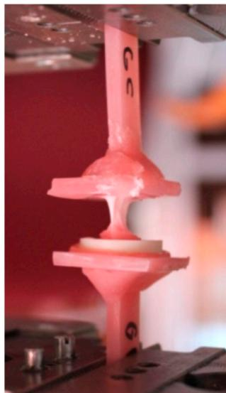
**Figure 1.** A sample during the test of the strength of the connection between the soft lining material and the acrylic resin.
