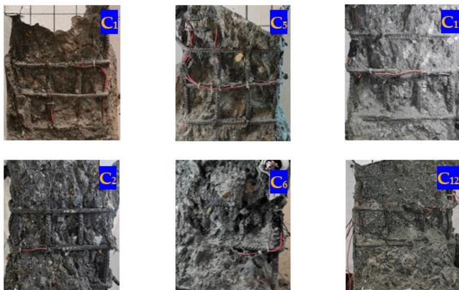
**Figure 6.** Concrete crushing modes of specimens with different stirrup configurations. (C<sub>1</sub>, C<sub>5</sub>, C<sub>11</sub> are the specimens with rectangular stirrup; C<sub>2</sub>, C<sub>6</sub>, C<sub>12</sub> are the specimens with complex stirrup).
