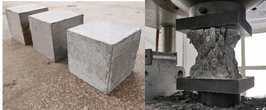
Figure 3. Concrete cubes and the failure mode of concrete tubes.
