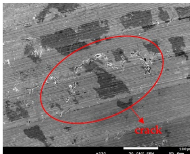
Figure 10. SEM morphology of the SCC in those samples with 0.1 \text{ g/m}^2 of chloride deposited after 7000 h of testing at RH = 70%.
