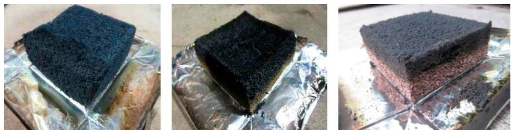
**Figure 7.** FR-EPS samples after the cone calorimeter test.
