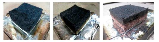
Figure 7. FR-EPS samples after the cone calorimeter test.
