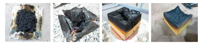
Figure 5. The specimen after 5 min of conducting the cone calorimeter method.
