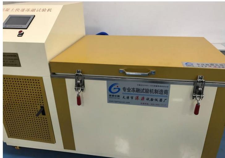
**Figure 2.** Automatic quick concrete freeze–thaw tester. Chinese in figure: Professional manufacturer of freeze–thaw testing machine, Tianjin Guanyuan Test Instrument Factory.
