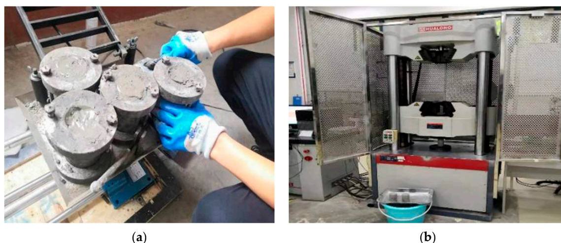
Figure 1. Pouring test piece site and rock mechanics testing machine. (a) On-site grouted specimens pouring. (b) Uniaxial experiment machine.
