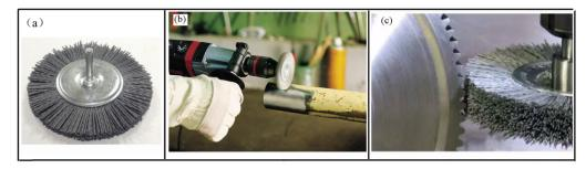
Figure 1. Abrasive filament brush (a); brush derusting (b); and grinding gear (c).
