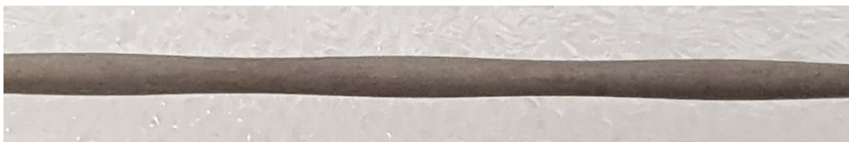
Figure 6. Macroscopic multi-neck effect observed for the sand casting of AZ91 (MgAl9Zn1) magnesium alloy extruded by the KOBO method with the processing degree of \lambda = 44.4 and the die rotation frequency f = 6 \text{ Hz} stretched at 300 °C with the speed \dot{\epsilon} = 10^{-4} \text{ s}^{-1} .
