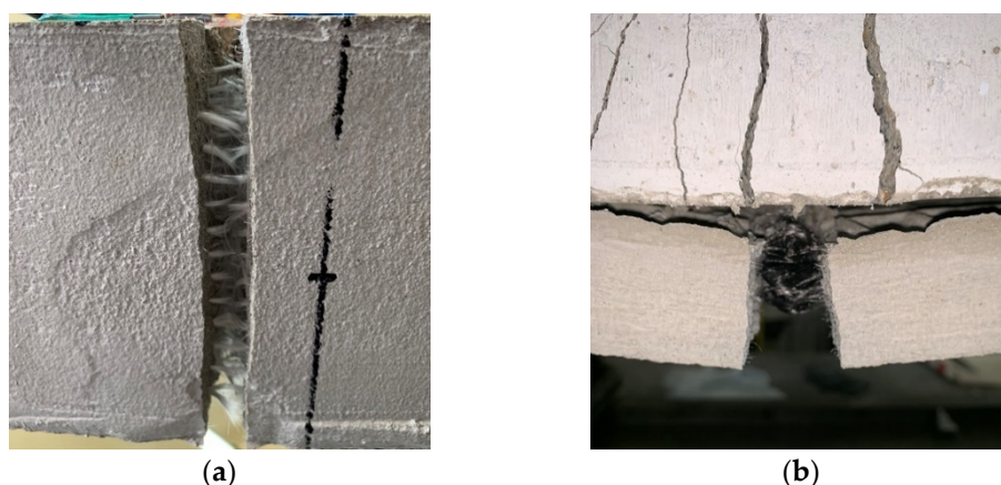
Figure 2. Failure modes: (a) Textile rupture; (b) IC debonding.
