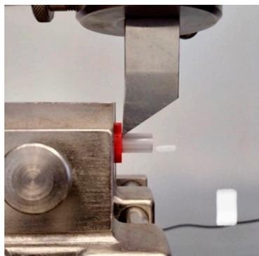
**Figure 5.** The setup for adhesion tests was performed using a shear test machine with a placed sample made of PLA as a bottom and TPU as a top cylinder.
