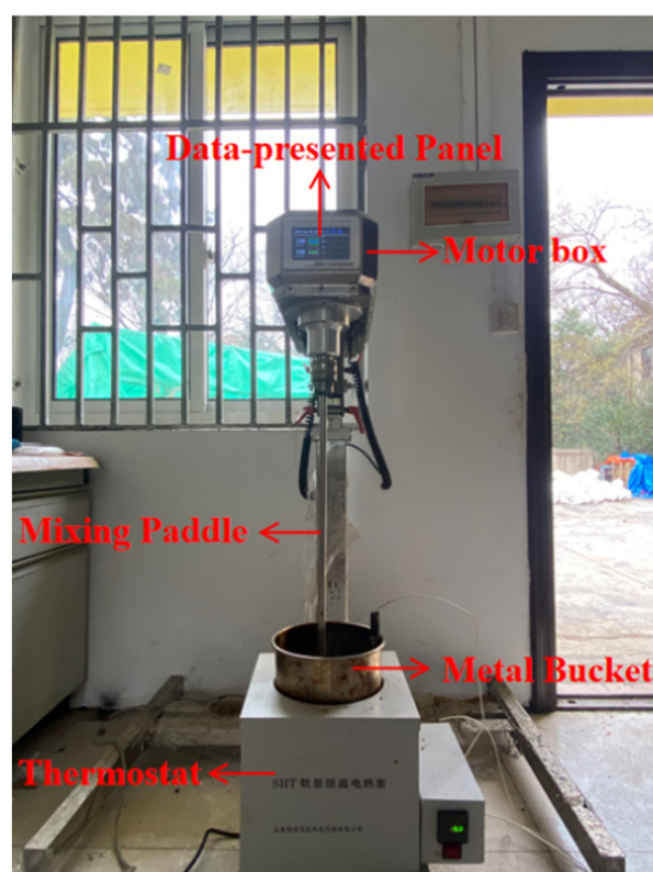
Figure 4. Mixing torque tester.
