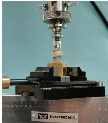
**Figure 6.** Crown set up for cyclic loading in the electro-dynamic testing system.
