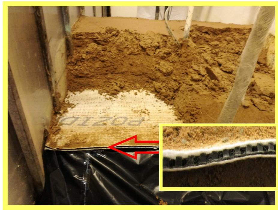
**Figure 1.** Drainage geocomposite with spatial structure in the form of an embossed core.
