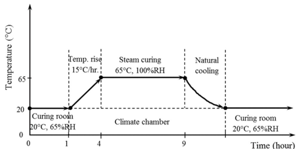
**Figure 1.** Schematic description of the steam curing process.
