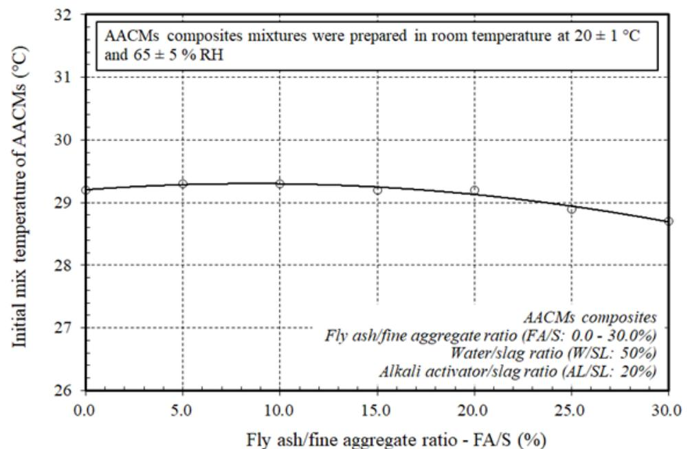
**Figure 2.** Effect of varying ratios of fly ash to fine aggregate on the initial mixing temperature of the AACMs composites.
