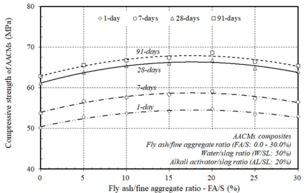
**Figure 4.** Effect of varying ratios of fly ash to fine aggregate on the compressive strength of the AACM composites.
