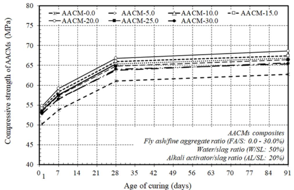
Figure 5. Compressive strength growth of AACM composites cured in steam at various ages.
