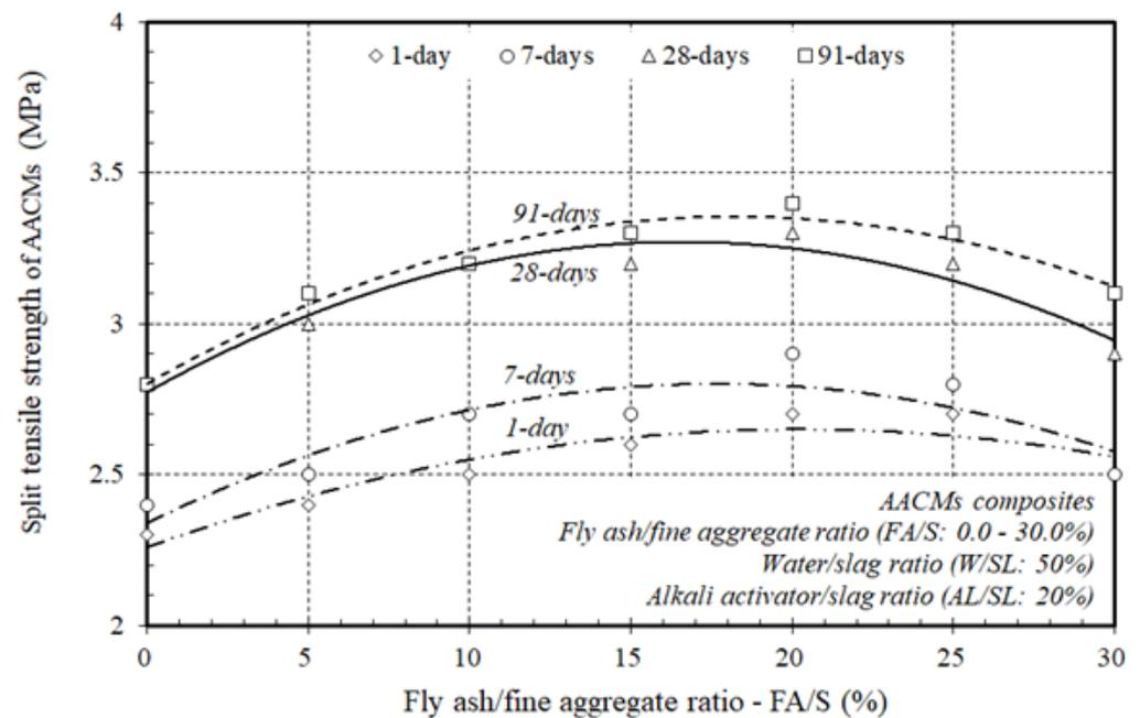
Figure 6. Effect of varying ratios of fly ash to fine aggregate on the split tensile strength of the AACM composites.
