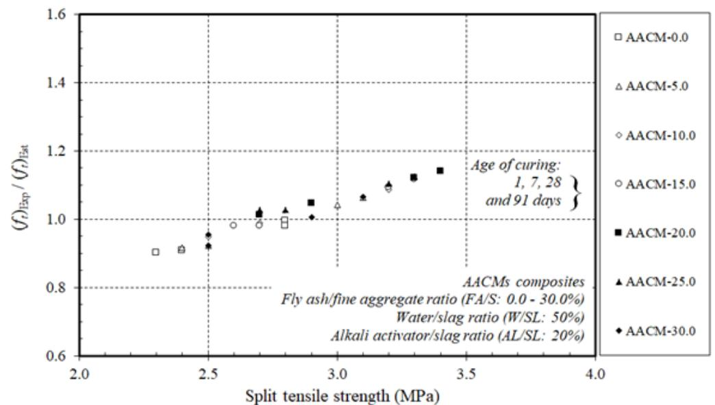
Figure 10. Ratio of experimental split tensile strength to split tensile strength estimated by ACI 318 of AACMs composites cured in steam.
