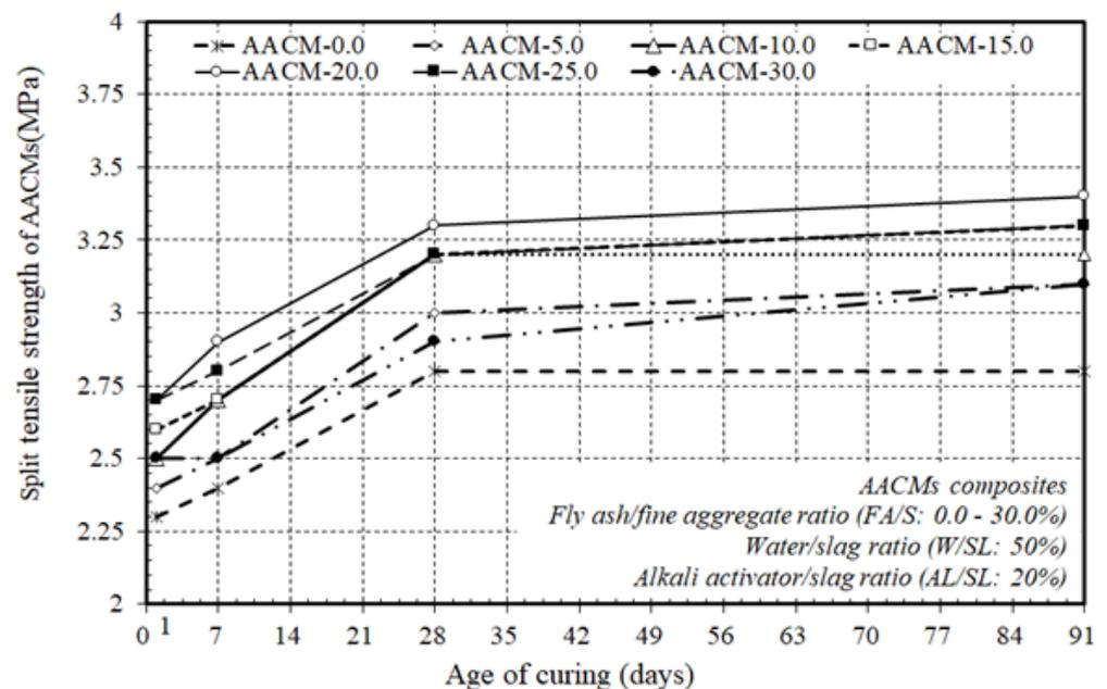
Figure 7. Split tensile strength growth of AACM composites cured in steam at various ages.
