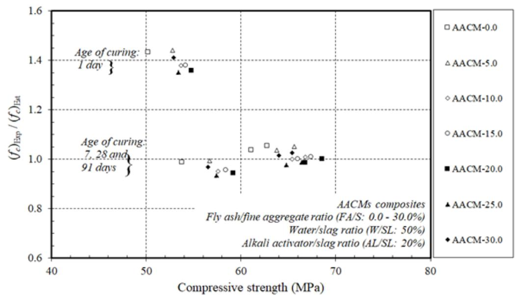
Figure 9. Ratio of experimental compressive strength to compressive strength estimated by ACI 209 of AACMs composites cured in steam.
