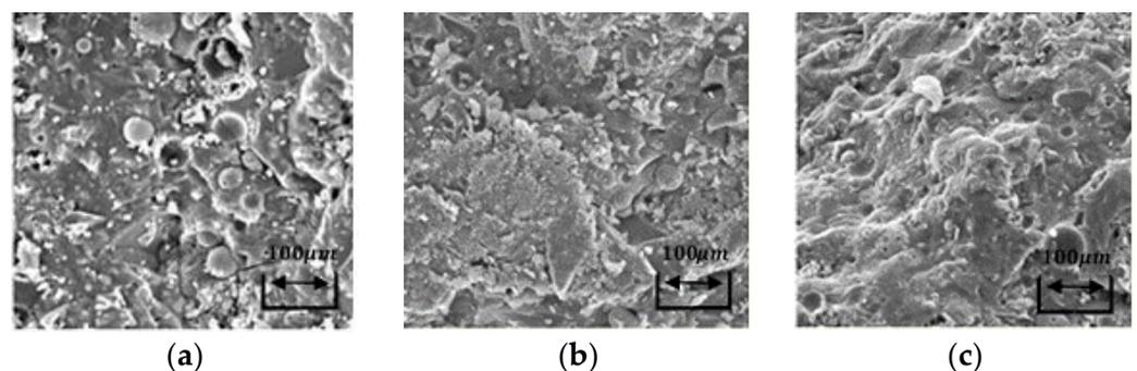
**Figure 8.** SEM micrographs of AACM composites cured in steam at: (a) 1 day; (b) 28 days; (c) 91 days.
