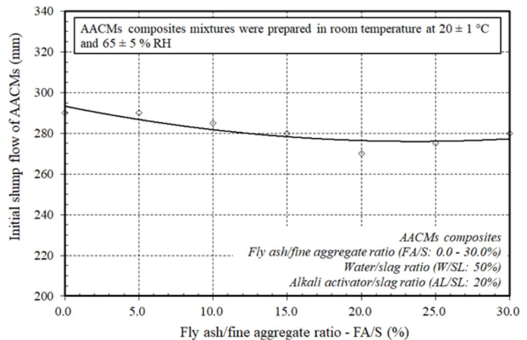
**Figure 3.** Effect of varying ratios of fly ash to fine aggregate on the initial slump flow of the AACMs composites.
