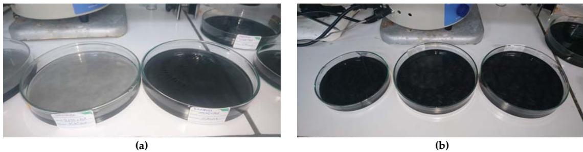
**Figure 3.** Suspension of PLA and CNTs (a) and suspension of PLA and GNP (b).
