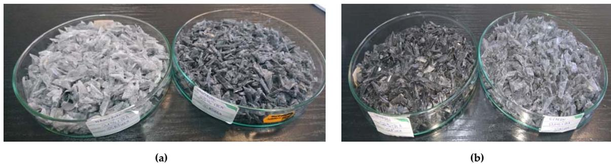
**Figure 4.** Composite PLA with CNTs in the form of cut pieces (a) and composite PLA with GNP in the form of cut pieces (b).
