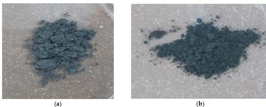
**Figure 1.** Graphene nanopowder (a) and carbon nanotubes (b) used as admixtures in PLA samples.
