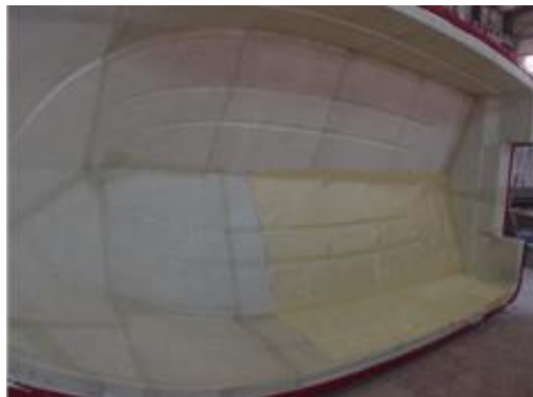
Figure 15. Laminate of hull structure.
