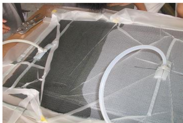
Figure 7. Manufacturing process of plate by resin transfer.
