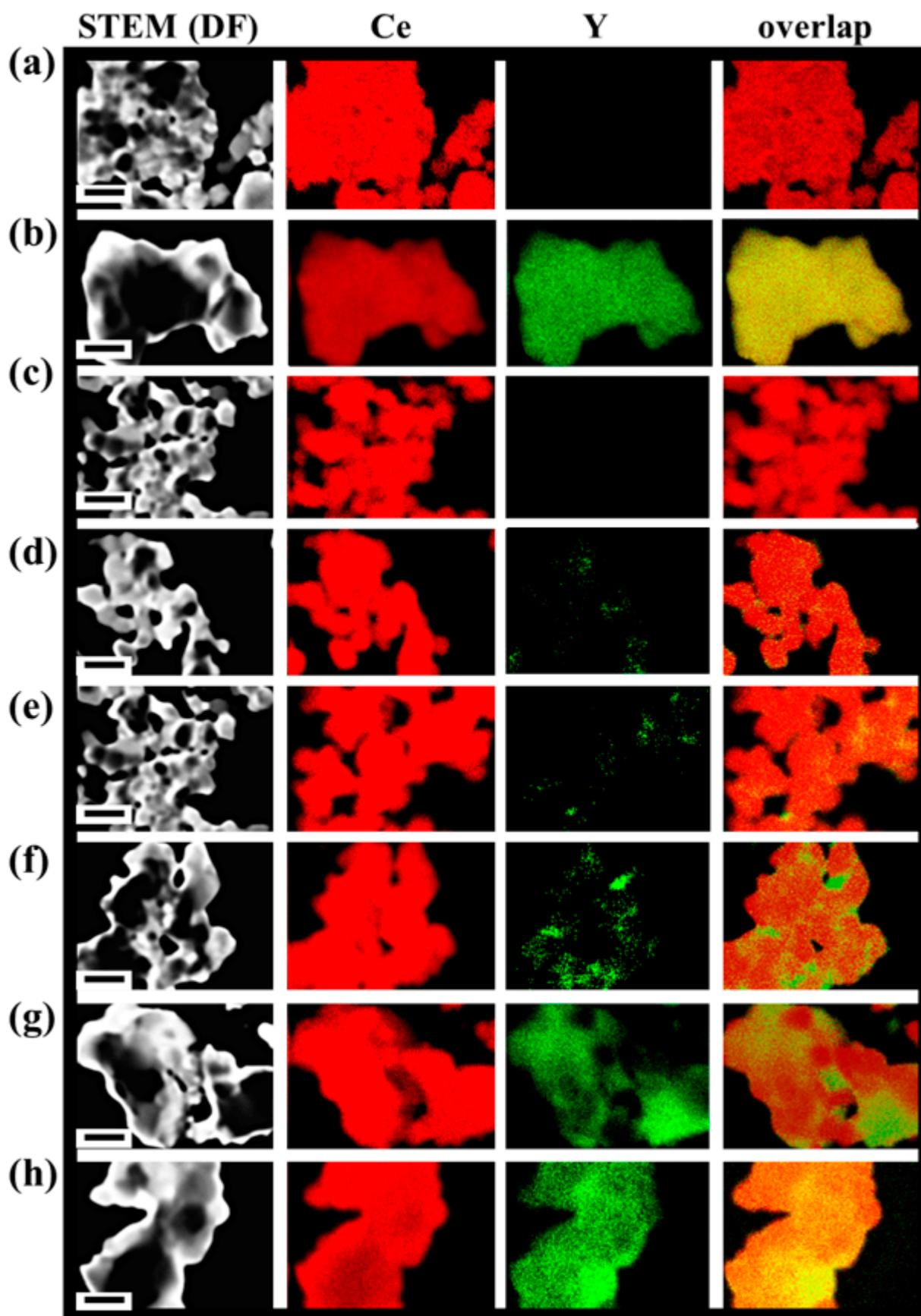
**Figure 2.** STEM/EDS mapping images of 1573K-Pure-CeO<sub>2</sub> (a), 1573K-CPT (b), 1273K-SSR (c), 1373K-SSR (d), 1473K-SSR (e), 1573K-SSR (f), 1673K-SSR (g), and 1773K-SSR (h). Scale bars are 400 nm.
