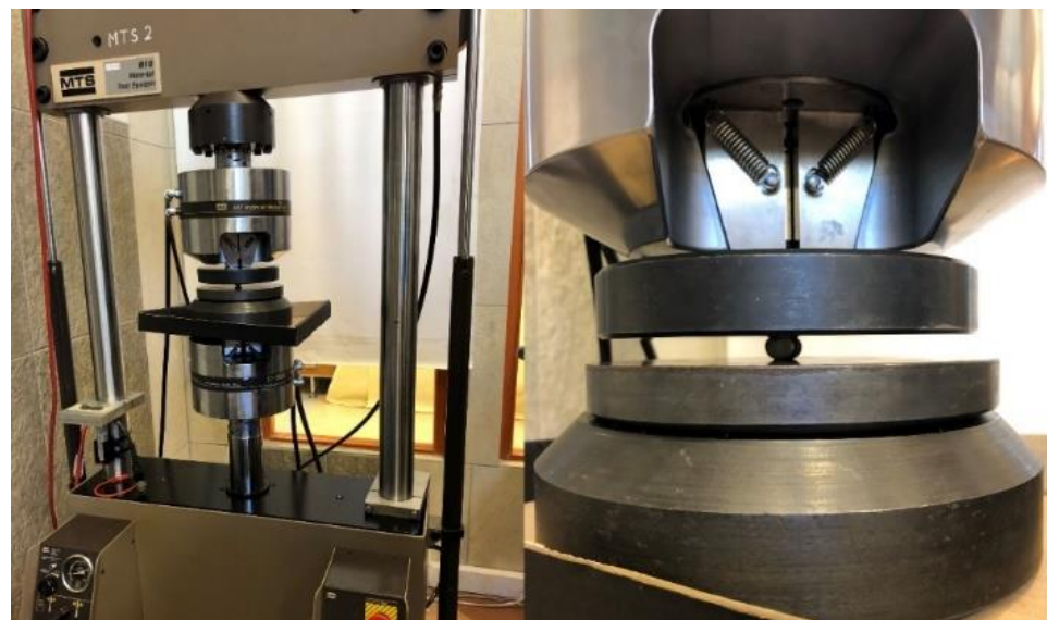
Figure 7. Specimen during the diametral compression test.
