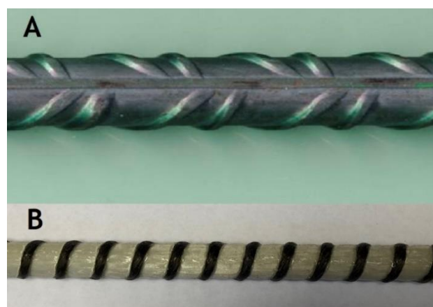
Figure 1. Concrete reinforcement–rebars subjected to mechanical testing; (A) B500SP steel, (B) GFRP rebar manufactured by Ankra company (Poland).
