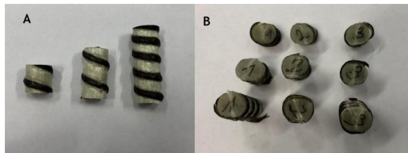
Figure 13. Samples used in diametral compression. (A) Before the test; (B) After compression test.
