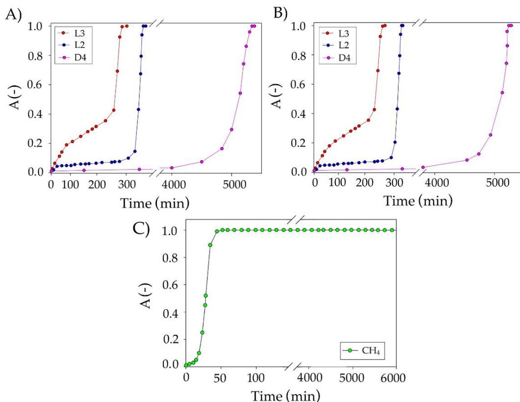
**Figure 14.** Experimental breakthrough curves of impurities absorption with TPABr:TEG (1:3) using (A) pure nitrogen and (B) mixture of nitrogen and methane at 2:1 volume ratio under optimum conditions, and (C) methane absorption curve using TPABr:TEG (1:3).
