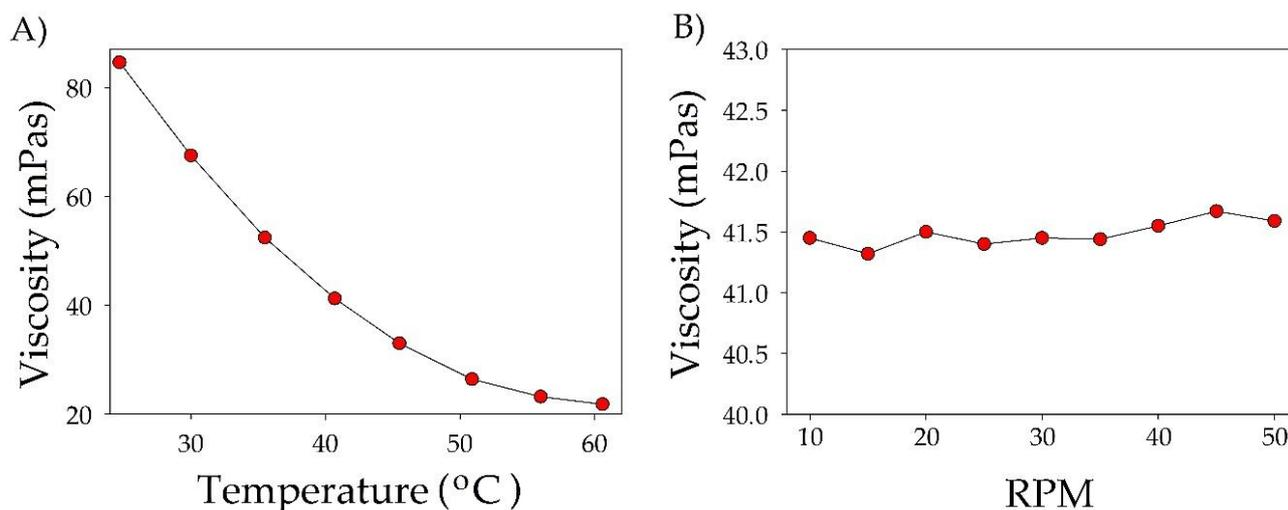
**Figure 9.** (A) Viscosity for TPABr:TEG (1:3) as a function of temperature in the range 25–60 °C. (B) Dependence of viscosity on turnover in the range 10–50 RPM in temperature 40 °C.
