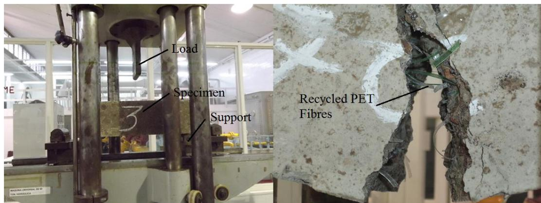
Figure 14. Flexural test.
