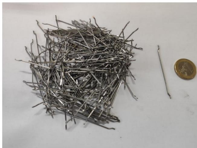
**Figure 2.** Hooked-end steel fibres used.
