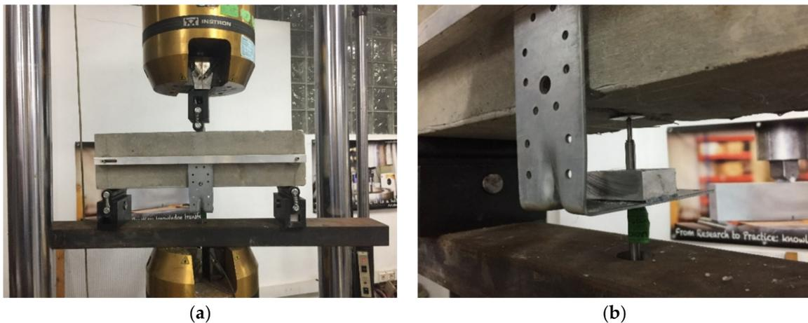
**Figure 3.** Flexural tensile strength test (a) and measurement of vertical displacement with a LVDT (b).
