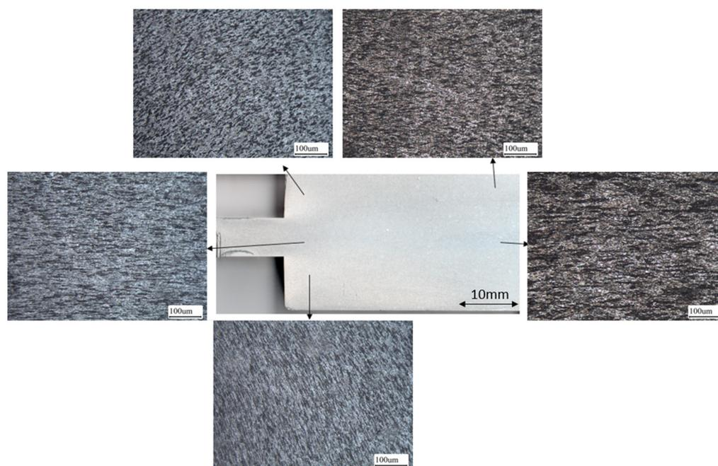
**Figure 3.** The macrostructures of the as-forged HF62 samples, showing the distribution of flow lines and deformation bands.
