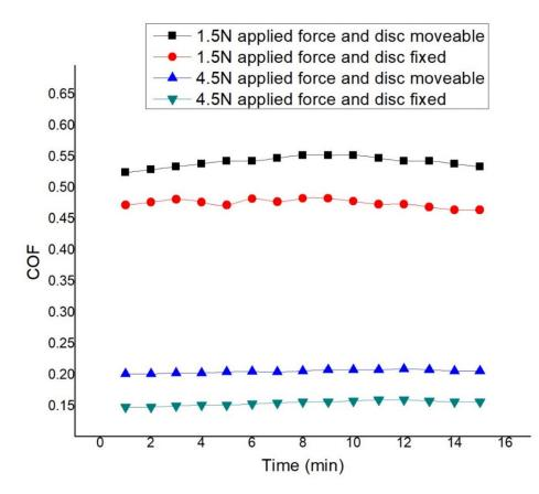
Figure 21. COF at 0.45 m/s disc, 0.2 m/s pin velocity, and dry condition.
