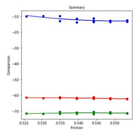
Figure 22. Regression model for COF at 0.45 m/s disc velocity, 0.2 m/s pin velocity, and dry condition.
