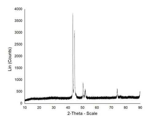
Figure 10. XRD analysis of coated mild steel sample.
