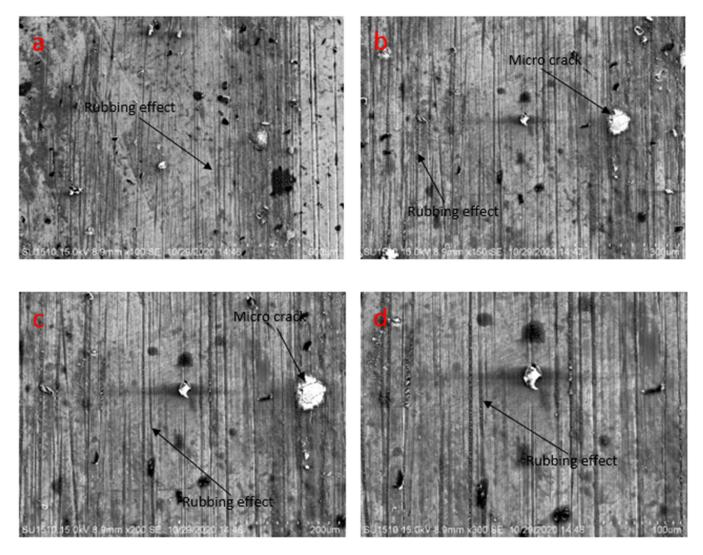
**Figure 20.** Scanning electron microscopy analysis of the sample after tribological test at 1.5 N applied force, 0.2 m/s pin velocity, and without lubricating condition (**a**) at 500  $\mu$ m, (**b**) at 300  $\mu$ m, (**c**) at 200  $\mu$ m, (**d**) at 100  $\mu$ m.
