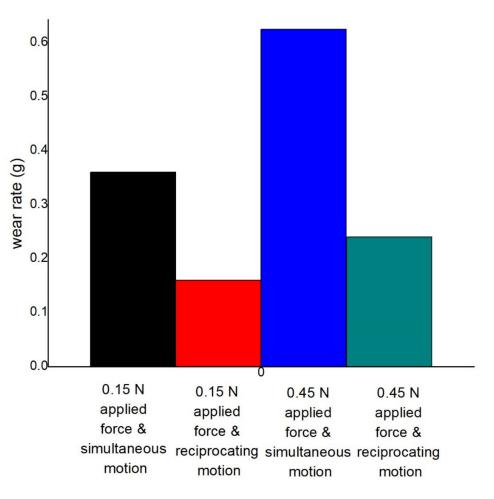
Figure 23. Comparison of wear rate at 0.45 m/s disc, 0.2 m/s pin velocity, and dry condition.
