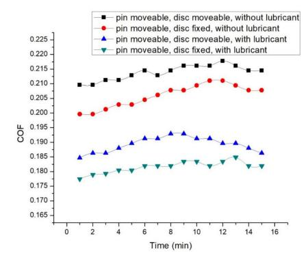
Figure 12. COF at 3.5 N normal load, 0.45 m/s disc, and 0.15 m/s pin velocity.
