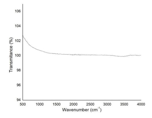
Figure 11. Fourier transform infrared ray analysis of coated mild steel sample.
