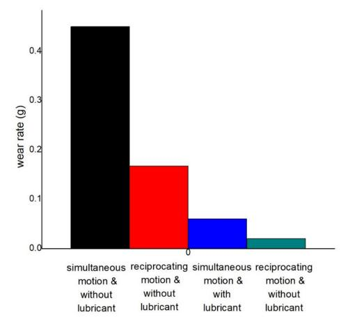
Figure 15. Variation of wear at 3.5 N load, 0.45 m/s disc, and 0.15 m/s pin velocity.
