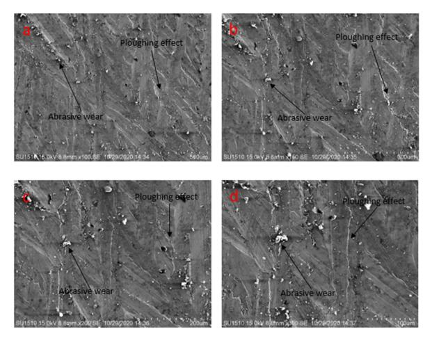
**Figure 24.** Scanning electron microscopy of the specimens after friction test at 4.5 N load, 0.2 m/s pin, 0.45 m/s disc velocity, and at dry condition (**a**) at 500  $\mu$ m, (**b**) at 300  $\mu$ m, (**c**) at 200  $\mu$ m, (**d**) at 100  $\mu$ m.
