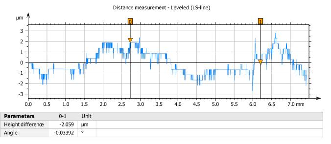
Figure 7. Analysis of the surface roughness of coated mild steel sample before the tribological test.
