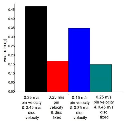
Figure 19. Wear rate comparison at 2.5 N load and dry condition.
