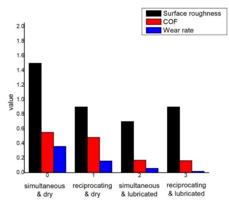
Figure 26. Surface roughness, COF, and wear rate comparison.
