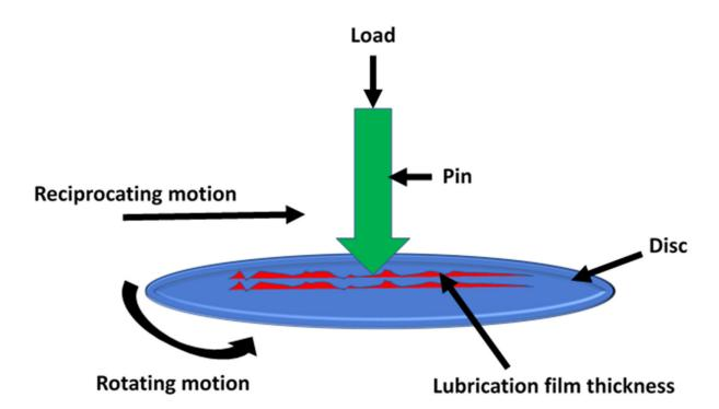
Figure 13. Lubrication mechanism for separating the mating surfaces.
