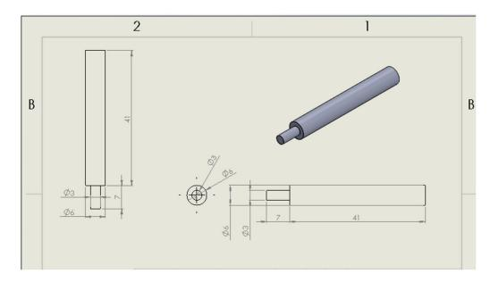
Figure 2. Projection view of pin sample [28].
