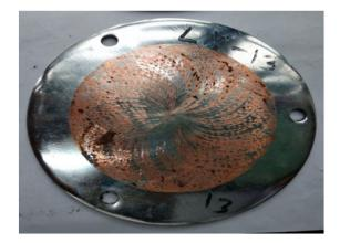
Figure 4. Disc after frictional analysis.
