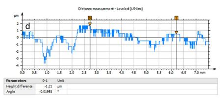
**Figure 25.** Roughness analysis of the sample at (**a**) simultaneous motion of pin and disc at dry condition, (**b**) reciprocating motion of pin at dry condition, (**c**) simultaneous motion of pin and disc at lubricated condition, (**d**) reciprocating motion of pin at lubricated condition.
