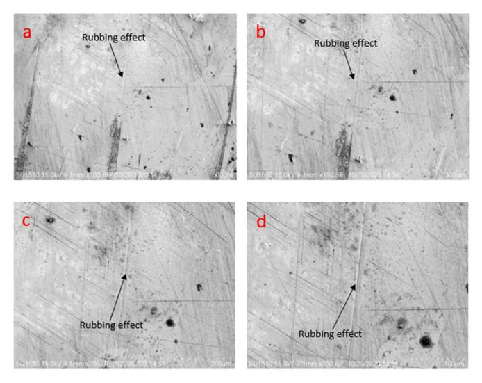
**Figure 16.** Scanning electron microscopy image of specimens' later friction test at 3.5 N load, 0.45 m/s disc, 0.15 m/s pin velocity, and lubrication (**a**) at 500  $\mu$ m, (**b**) at 300  $\mu$ m, (**c**) at 200  $\mu$ m, (**d**) at 100  $\mu$ m.
