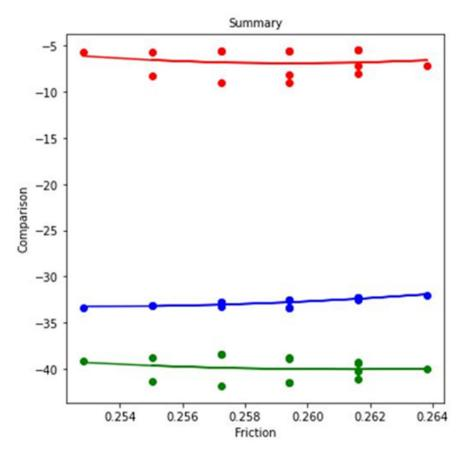
Figure 18. Regression model for COF at 2.5 N load and dry condition.
