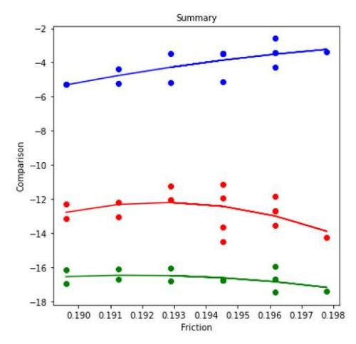
Figure 14. Regression model for COF at 3.5 N applied force, 0.45 m/s disc velocity, and 0.15 m/s pin velocity.
