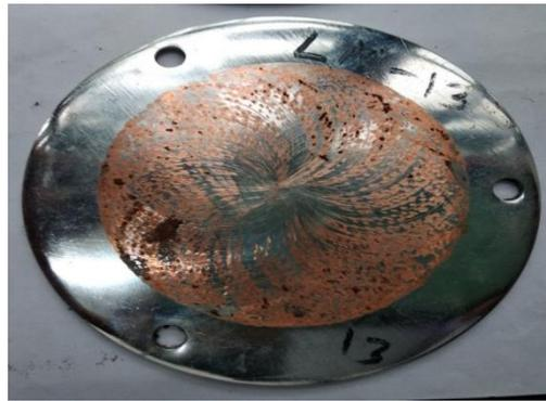
**Figure 4.** Disc after frictional analysis.
