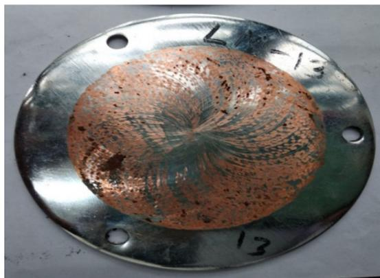
**Figure 4.** Disc after frictional analysis.
