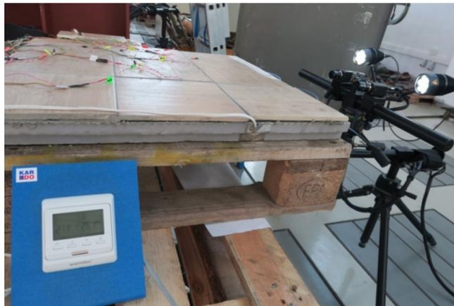
**Figure 11.** Aramis system test stand for measuring LFS displacements.
