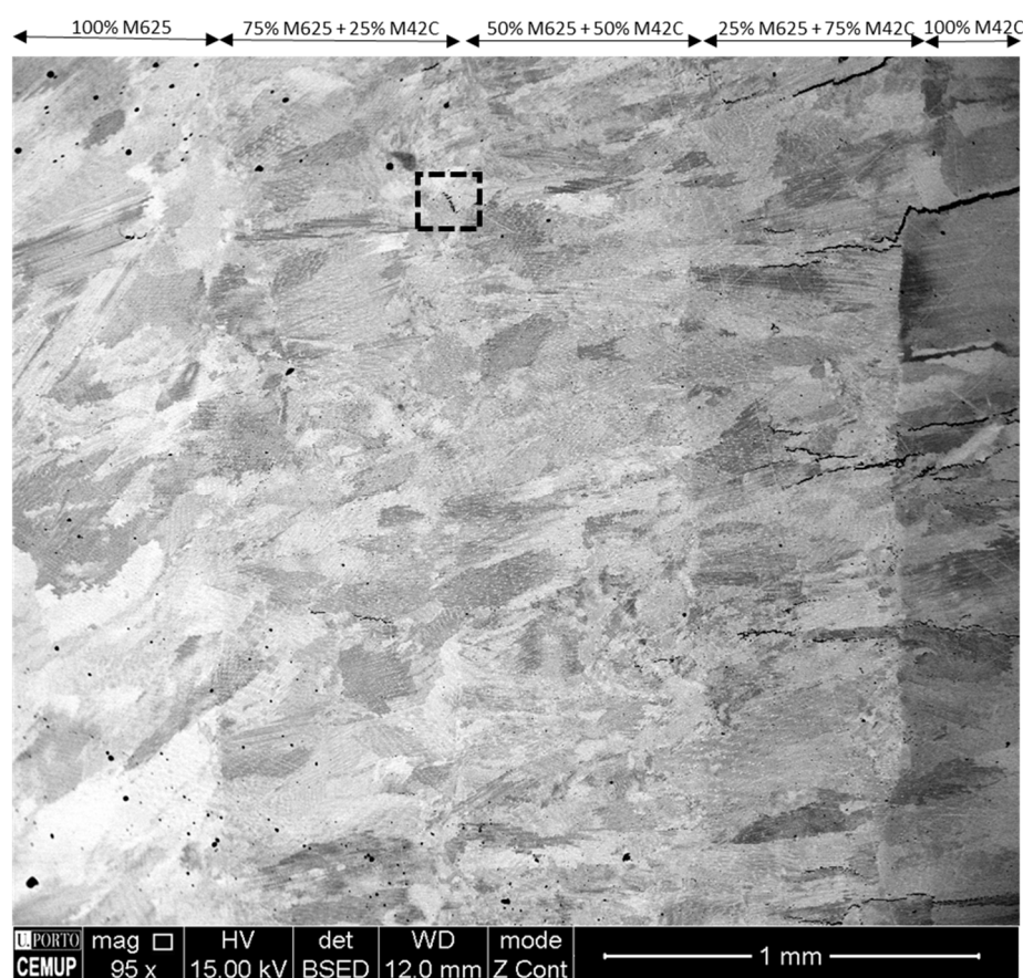
Figure 2. Microstructural evolution across the longitudinal section of the FGM specimen without PHT, SEM/BSE image.
