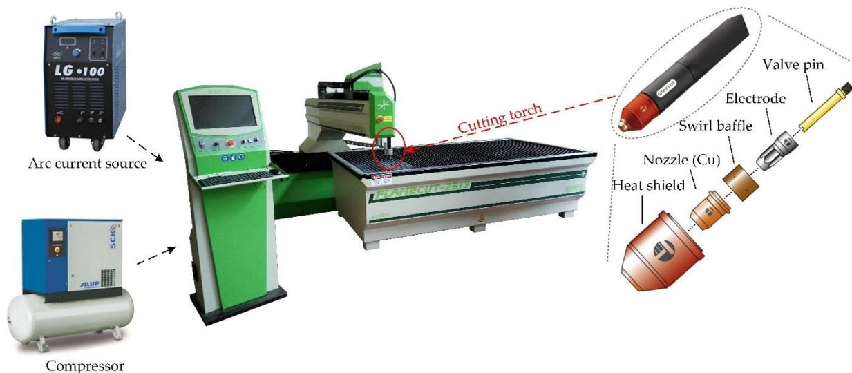
**Figure 1.** CNC machine FlameCut 2513, cutting torch, arc current source, and compressor.
