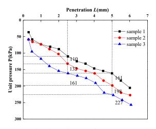
Figure 6. The relationship curve between unit pressure and penetration.
