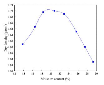
Figure 5. Compaction test curve.
