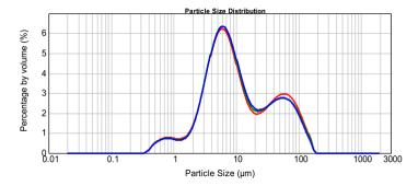
Figure 4. Particle size distribution curve of manganese slag.
