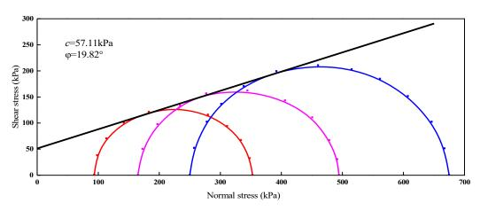
Figure 10. Envelope of consolidated undrained shear strength.
