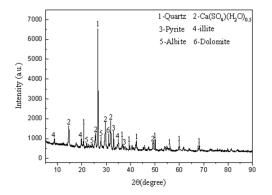
Figure 1. XRD pattern of manganese slag.
