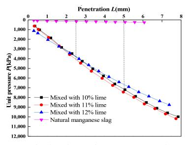
**Figure 8.** The relationship curve between unit pressure and penetration of lime-solidified manganese slag.
