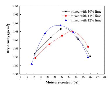
Figure 7. Compaction curve of lime-solidified manganese slag.
